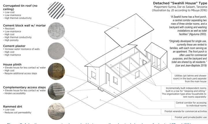
Figure 2. Adaptive measures implemented to improve the physical structure of a typical "Swahilli" house typology in Dar es Salaam, Tanzania. Illustration inspired by data from Mbuya 2016
