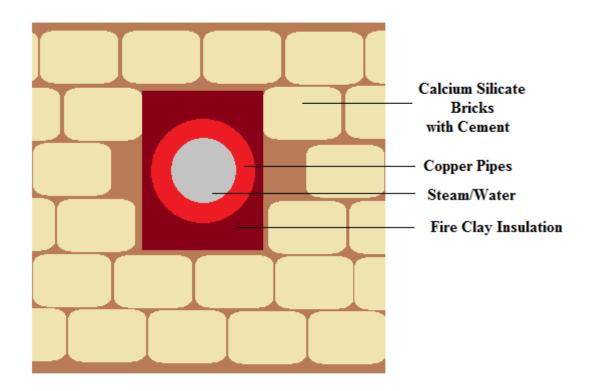
For a particular corner in the Salt Chamber the Airgap insulation is shown below. The Copper pipe in this section is free from the cavity to facilitate conduction for heat exchange.
