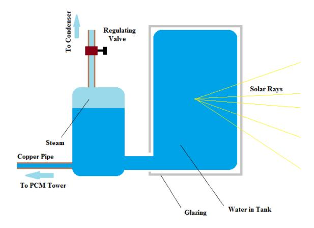
The tank is kept at the ground level so that the steam generated will automatically go up to the condenser without the help of a pump. However for practical feasibility of cooking process we may encounter the need for a pump for faster circulation. The Copper pipes help in the convection of heat to the PCM tower.
