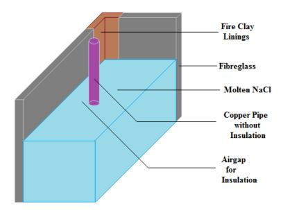
The inner surface of the wall is lined by Fire Clay Linings to resist the high temperature thus generated.
