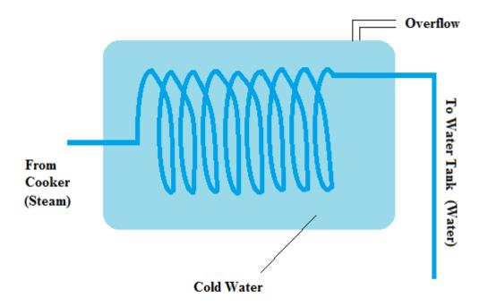
This tank is unpressurised and has an outlet for coolant overflow.
